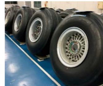
Final line of the wheel overhaul
