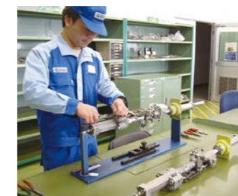
Servo cylinders and actuators control the blades of rotary-wing aircraft using hydraulic pressure.
