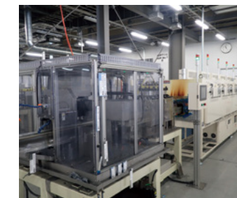
Molding line for ADvanced pultrusion (ADP)
