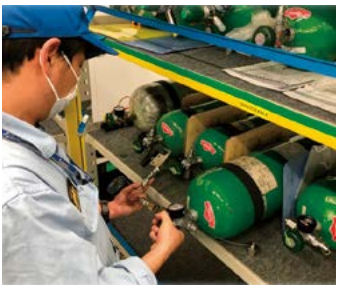
Overhaul of High pressure gas cylinder
