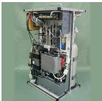
CME (Continuous Carbon Dioxide Measuring Device)
