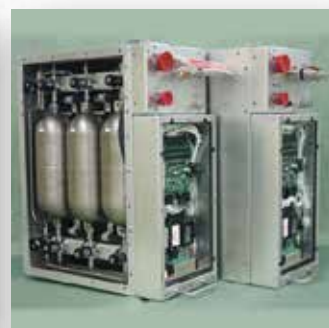
ASE (Automatic Atmospheric Sampling Device)
