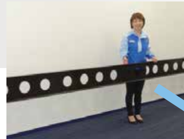
CFRP manufactured with the ADP method
