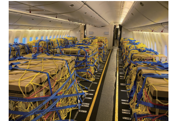
Passenger cabin after retrofitting We fit mechanisms to secure cargo to the floor, enabling it to be carried in the optimal configuration. The cargo capacity is increased by 12% compared to a regular Boeing 777-300ER aircraft. The STC was swiftly obtained, enabling the conversion from passenger cabin to cargo hold to be achieved in a short period of time.
