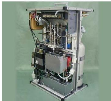
CME (Continuous Carbon Dioxide Measuring Device)
