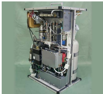
CME (Continuous Carbon Dioxide Measuring Device)
