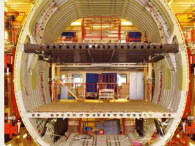
CFRP upper-deck floor cross beams, manufactured in the ADP manufacturing method, for the Airbus A380 (Photo courtesy of Airbus)
